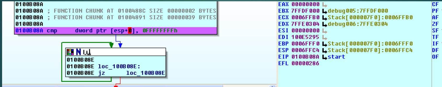
Osiris – disassembled execution trace with stack, registers and flags
