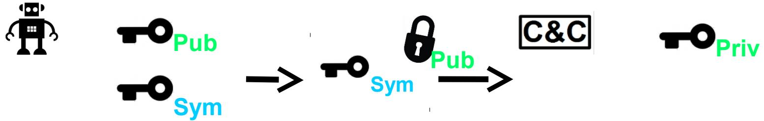
3. The C&C obtains the Symmetric Key and sends Encrypted Commands to the Bot
